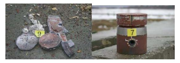
Figure 5: Bullet impact test results on HV-XRT 2. Left: violent reaction. Right: no reaction.
